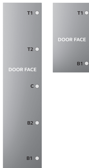
DRILLING POSITION HINGED RIGHT
